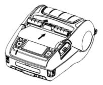
2. Slide the peel bar back then pull the paper.
